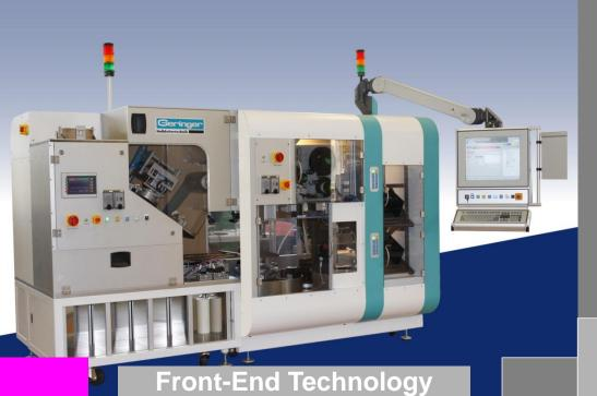
The FWL 100 is a flexible, fullyautomatic in-line frame and wafer laminating system for wafers up to 6" in diameter. It is the ideal solution when it comes to laminate films and very thin wafers made from brittle materials tension free at high speed and with unprecedented precision. The modular design, state-of-the-art vacuum lamination technology, user friendly machine/operator interface and material tracing system make the FWL 100 the lamination system of your choice.
